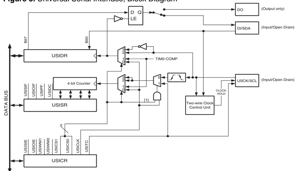
**Figure 4.** Two-wire Mode Operation, Simplified Diagram
