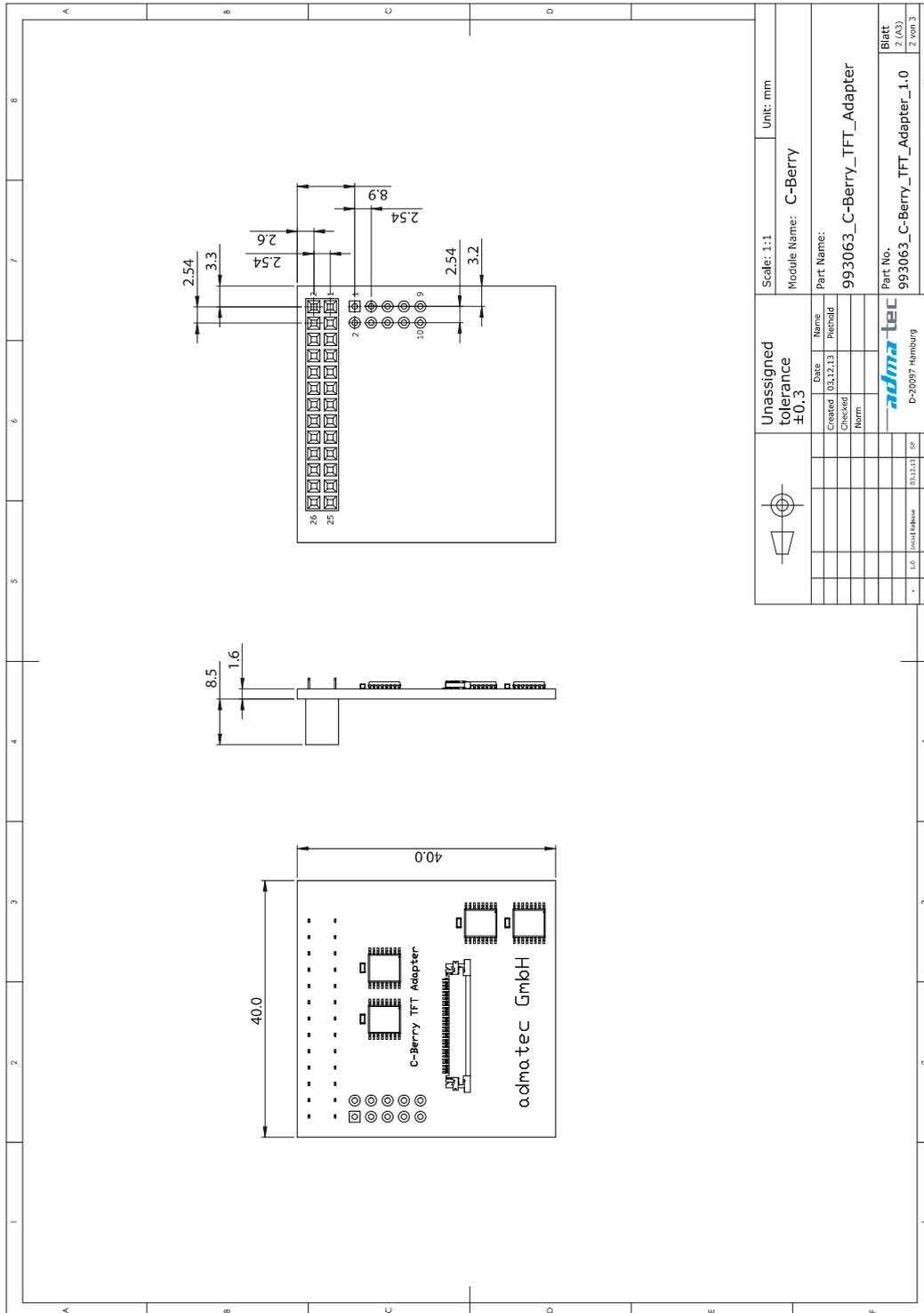
Fig 12.2: Drawing of C-Berry TFT Adapter
