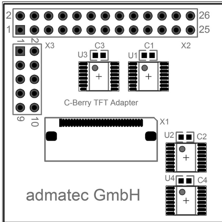
Figure 7.2 : PCB for C-Berry TFT Adapter
