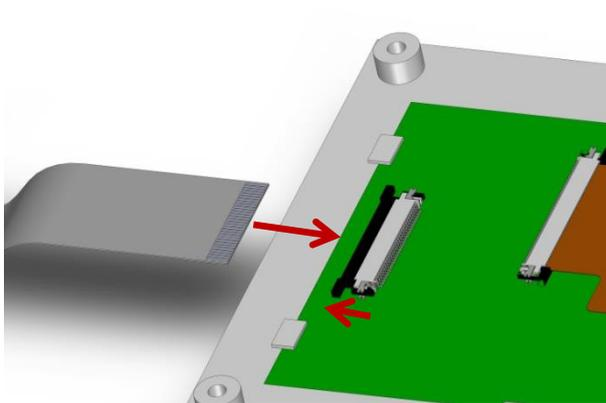
**Figure 11.1: Connect FFC with TFT Module**
