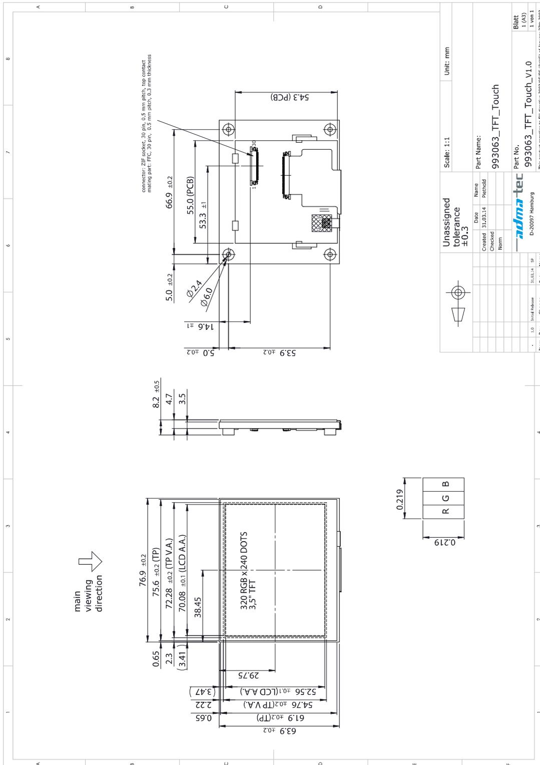
Fig 12.1: Drawing of TFT Module
