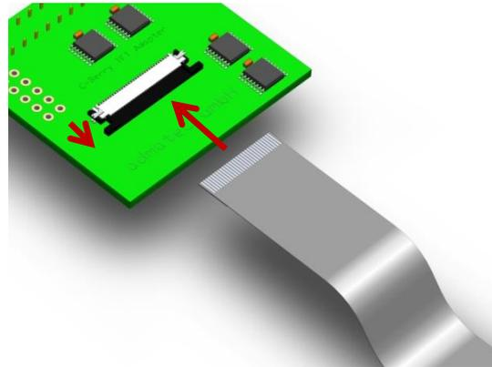
**Figure 11.2: Connect FFC with C-Berry TFT Adapter**
